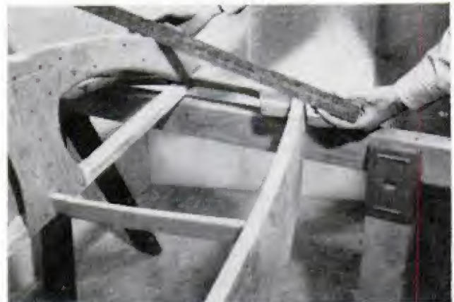
YARDSTICK is used to simulate planking which must rest on both keel and chine and not just one edge
